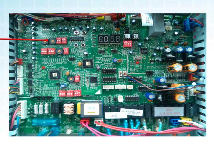
If part of indoor units in one system power down when the unit is running, the outdoor units will stop and show fault code "H7"
